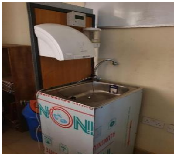
Figure 8: Side view of the visitor counter with automatic hand cleaning station
