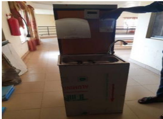
Figure 7: Front view of the visitor counter with automatic hand cleaning station
